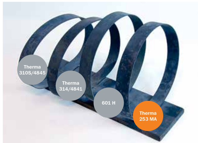
Therma 310S/4845 and Therma 314/4841 rings collapsed due to their own weight. 1000 °C/1830 °F, 35 hours, 1 mm/0.04 in thickness.
